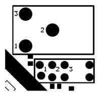
For this purpose, the negative pole must be connected to the ground connection of the socket (pin 2 or 3, top), the positive connection to pin 1 of the socket, or to pin 2 of the switch (bottom, if present). The above given voltages for the switching points of the amplifiers apply.
