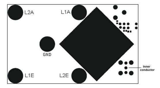
The two receiving loops must be routed with their ends to holes L1A - L1E (first loop) or L2A - L2E (second loop). The holes are 4.3 mm in size and thus allow connection by means of M4 screws. To protect the printed circuit board, it is essential to place shims!
