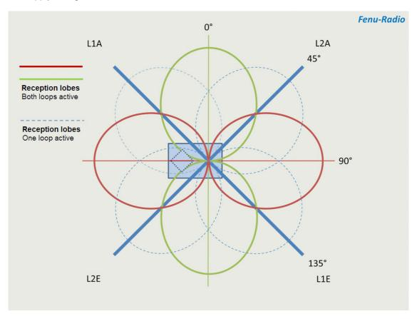
As of version 4E, the loops are not only controlled by an analogue DC voltage, but also by digital modulation of the remote supply voltage (logically negative RS-232 signal (start bit = increased supply voltage, stop bits = supply voltage). In this case, a data word is sent from a control unit (modulator) to the antenna. This data word contains a command for setting the receiving direction. Depending on the version, different settings are possible:
