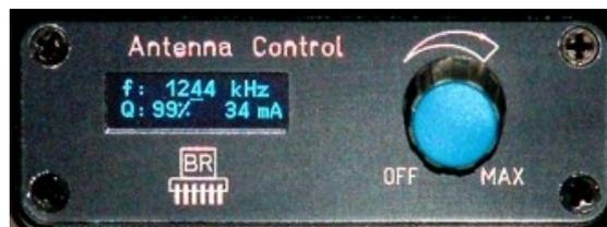
The set values for the frequency "f" and the quality factor "Q" as well as the measured value for the antenna current are visible in the display. The frequency can be set in 1, 10 and 100 kHz steps with the rotary encoder. To do this, a cursor (line under a number) can be moved to the desired position with the rotary encoder pressed. If the cursor is moved under the last digit of the Q factor, this value can be changed.
