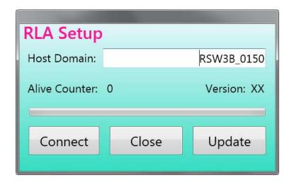
In the text field "Host Domain" (called "RSW Name\_S/N" in newer versions) the address under which the RAP1 can be reached by the program must be entered. Depending on how it is coupled with other devices (computer, router, ...) (see below) and the connections via which the program can access these devices (LAN connection, Internet, WiFi Direct, cellular network, ...) different possibilities exist. 2 basic variants exist:
