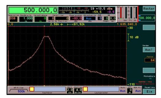
Setting 0.5 MHz: The filter curve (slightly overcritical coupling) is just under 500 kHz with the left side.
