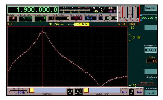
Setting 1.9 MHz: The filter curve (end of the 1st range, subcritical coupling) is steepened in the higherfrequency range by an additional notch filter and is therefore almost symmetrical in the linear frequency representation.
