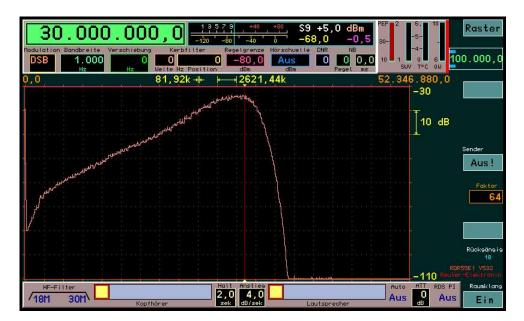
Setting 30 MHz: The filter curve becomes relatively wide above approx. 15 MHz (decreasing quality of the components used). A steep low-pass filter works at the upper end (RDR55 receiver), so that the upper edge can no longer be displayed correctly in the spectrum.
