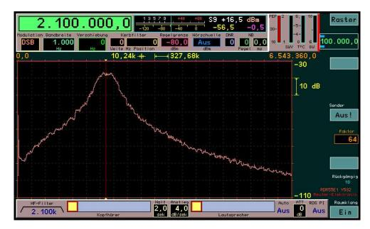
Setting 2.1 MHz: At the beginning of the 2nd range, again flat coupling (slightly overcritical).
