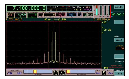
Intermodulation at 7.1 MHz: Despite active amplification and relatively small filter components as well as fully electronic tuning (using many switched semiconductors), the RAP1 only generates a small amount of IM (IP3 of the measurement in the picture approx. +23 dBm). As long as the downstream receiver does not have a significantly higher IP3, it is very unlikely that the reception will be impaired by the IM distortions of the RAP1.
