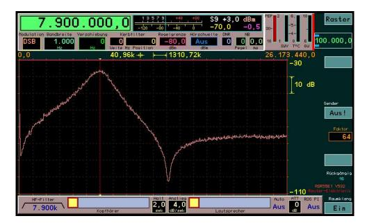
Setting 7.9 MHz: At the end of the 2nd range again subcritical coupling with additional notch filter.
