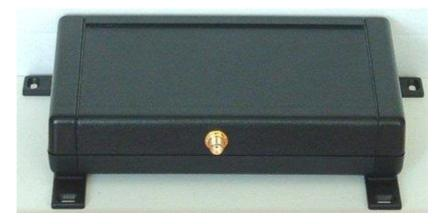
The housing of the RFA1B is slightly smaller than that of the 1A, has no special front panel and is waterproof. A waterproof (only when connected!) SMA socket is installed as the HF connection. This means that the antenna can be installed outdoors. The coaxial cable with plug should then also be suitable for outdoor use. In the case of permanent external installation, the connection point should be securely sealed with vulcanizing tape or similar.
