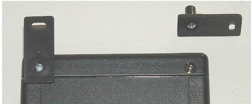
The housing feet are simply pushed on as standard and clamp in the holes of the housing screw connection.
