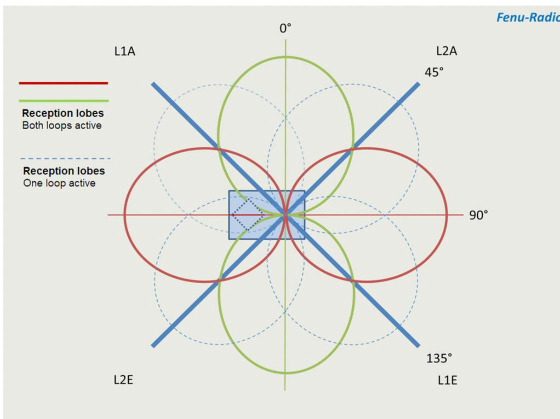
As of version 4E, the loops are not only controlled by an analogue DC voltage, but also by digital modulation of the remote supply voltage (logically negative RS-232 signal (start bit = increased supply voltage, stop bits = supply voltage)). In this case, a data word is sent from a control unit (modulator) to the antenna. This data word contains a command for setting the receiving direction. Depending on the version, different settings are possible:
