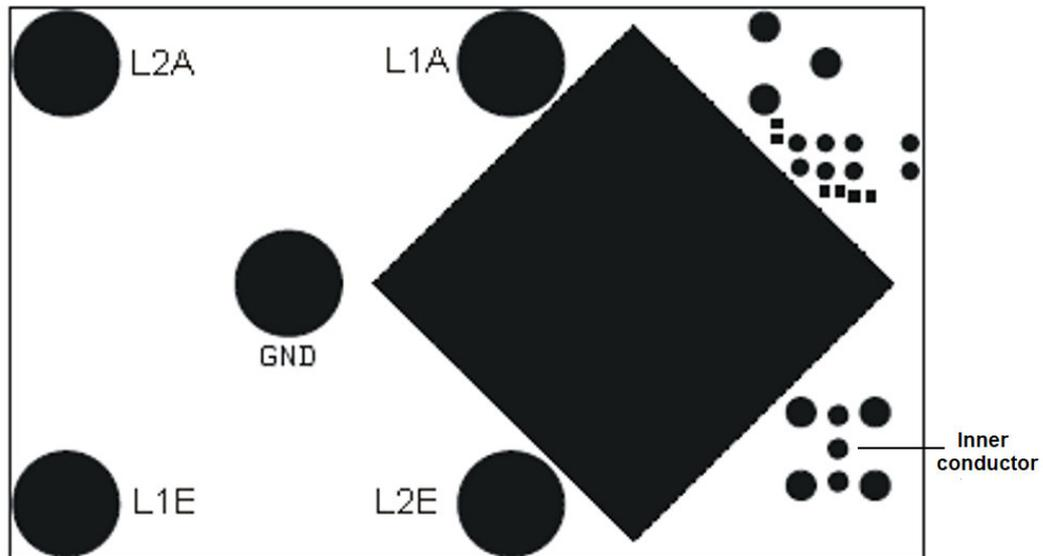
The two receiving loops must be routed with their ends to holes L1A - L1E (first loop) or L2A - L2E (second loop). The holes are 4.3 mm in size and thus allow connection by means of M4 screws. To protect the printed circuit board, it is essential to place shims!
