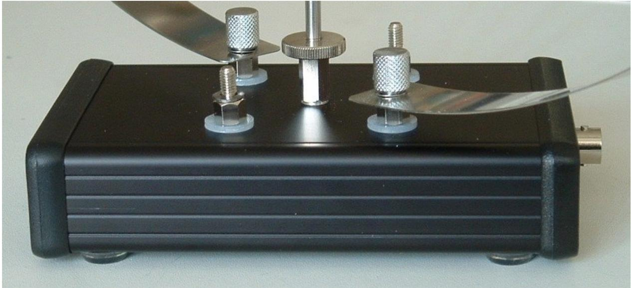
**Connection bolt of the amplifier with an installed steel strip**
