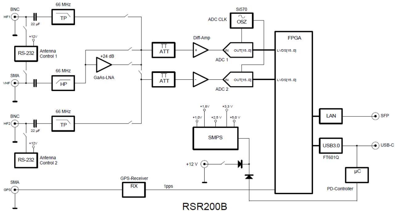
The analogue signals fed in at the inputs are digitized after filtering and amplification by two analogue-to-digital converters (ADCs): each with 16-bit amplitude resolution. The ADCs can be operated with an adjustable clock rate of 70 - 200 MHz. The digital output signals are fed into a highly integrated programmable circuit (“FPGA”: Field Programmable Gate Array). This pre-processes the data and controls various interfaces for transmission to a PC.
