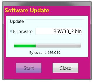
The "Firmware" field is initially empty. With a double click / tap on it, the program searches for transferable files. These files must always have the extension. Bit and be located directly in the ExtIO\*.DLL folder. If there are several \*.Bit files in the folder, the first one that can be found (depending on the arrangement of the files in the folder) is used. To avoid confusion, there should always be only one update file in the folder, namely exactly the (new) firmware to be transferred.
