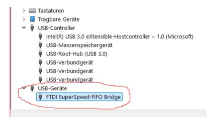
The new "WU" driver can be specified in the Device Manager after opening the properties for the previous FT601 entry under "USB controllers." After updating the driver, only FTD3XXWU.DLL (and the associated ExtIO RSR200B210.DLL) can be used for the SDR program. The old DLLs can be deleted once the new driver is running reliably.
