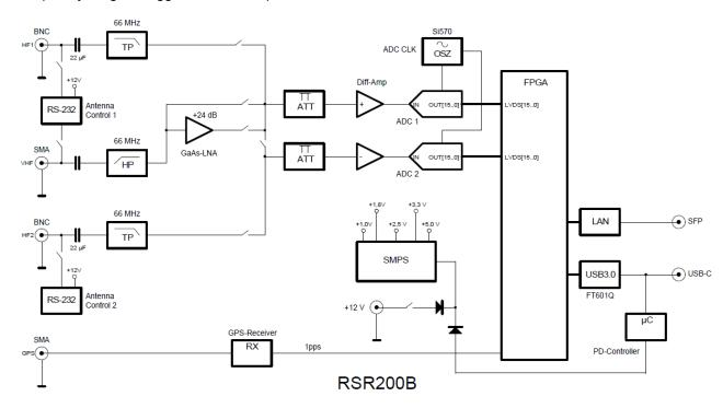
The analogue signals fed in at the inputs are digitized after filtering and amplification by two analogue-todigital converters (ADCs): each with 16-bit amplitude resolution. The ADCs can be operated with an adjustable clock rate of 70 - 200 MHz. The digital output signals are fed into a highly integrated programmable circuit ("FPGA": Field Programmable Gate Array). This pre-processes the data and controls various interfaces for transmission to a PC.
