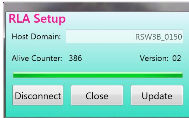
When the antenna is connected (note "RLA connected!" at the top right of the main program window), an "Alive Counter" (activity counter) counts the data that is constantly exchanged between the program and the control unit (at least 2 data packets per second). To the right of this, the firmware version contained in the RSW3 is displayed (see below under "Update").
