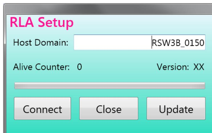
In the text field "Host Domain" (called "RSW Name\_S/N" in newer versions) the address under which the control unit can be reached by the program must be entered. Depending on how it is coupled with other devices (computer, router, ...) (see below) and the connections via which the program can access these devices (LAN connection, Internet, WiFi Direct, cellular network, ...) different possibilities exist. 2 basic variants exist:
